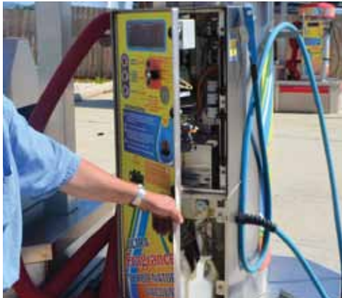
Step 2: Open up the front face doors of the unit.
