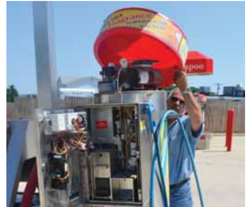
Step 4: Remove the Dome from the top of the unit.
