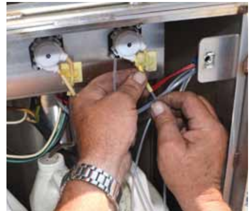
Step 15: Reconnect the three feed hoses to the Peristaltic Pumps. Once this is done, turn the power back on to your unit and test it before reassembling the entire unit. You'll want to ensure that fragrance is coming out for all three fragrance selections.
