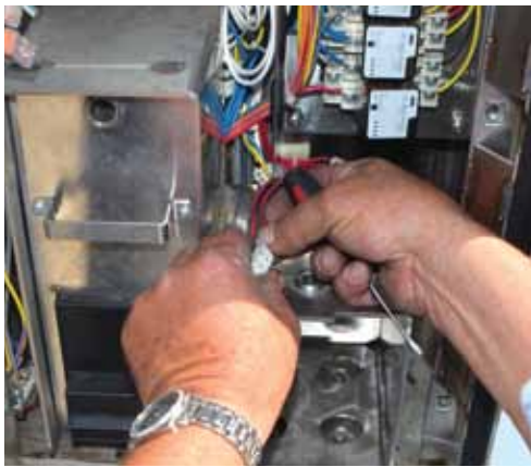
Step 8: Once located, unhook the wires of the old handle from the connector.
