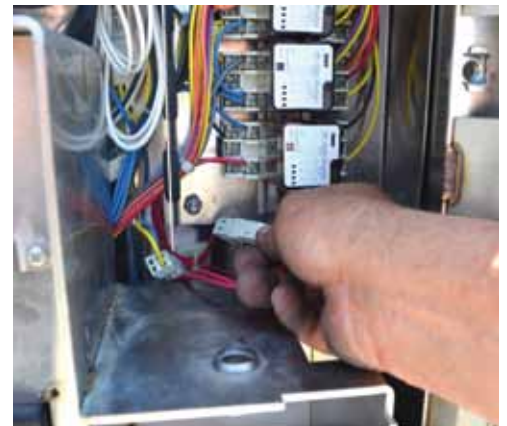
Step 7: Remove all the tie wraps from the power lines. Locate Connection #14 on an Adams Combo Unit, these are the wires for the button on the spray gun.
