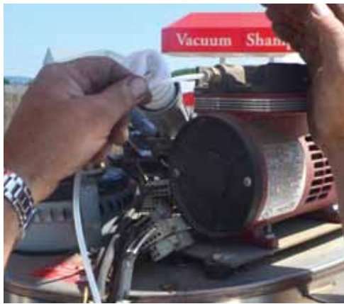
Step 9: Remove the Air Line from the compressor on top of your unit. Once the wires and air line from your old hose are disconnected, remove the old hose completely from your unit.
