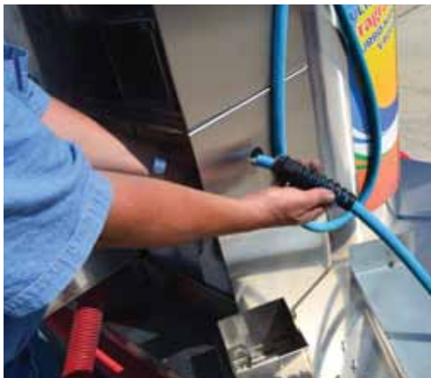
Step 5: Loosen up the Lock Nut on the hose from the inside of the cabinet.
