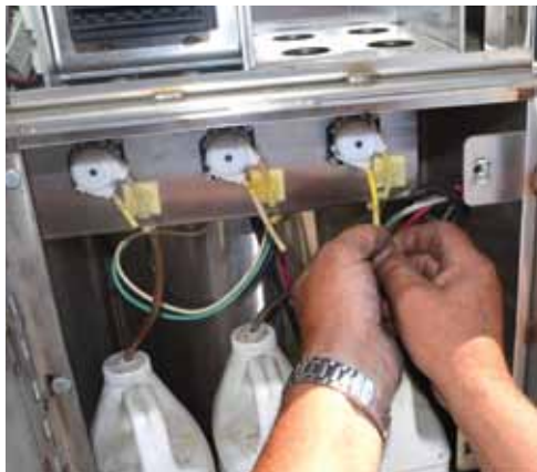
Step 6: Unhook the three Pick-Up Tubes from the Peristaltic Pumps.
