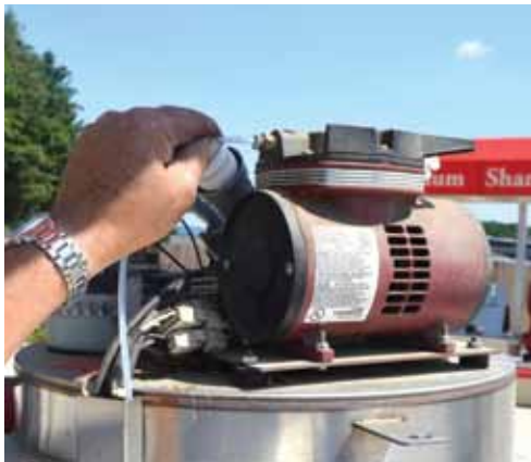
Step 13: The Air Hose will continue up through the channel until it comes out at the top. Cut off any excess tubing and attach to the air compressor.
